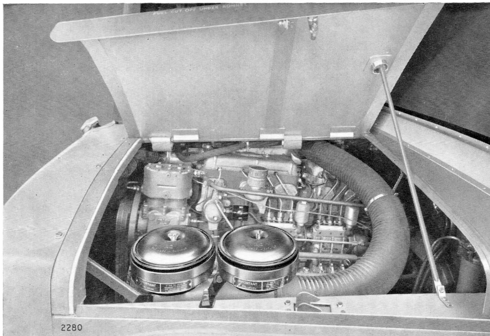
Fig. 51. Under-bonnet Installation of Twin Oil Bath Type Air Filter on a Passenger Carrying Vehicle
